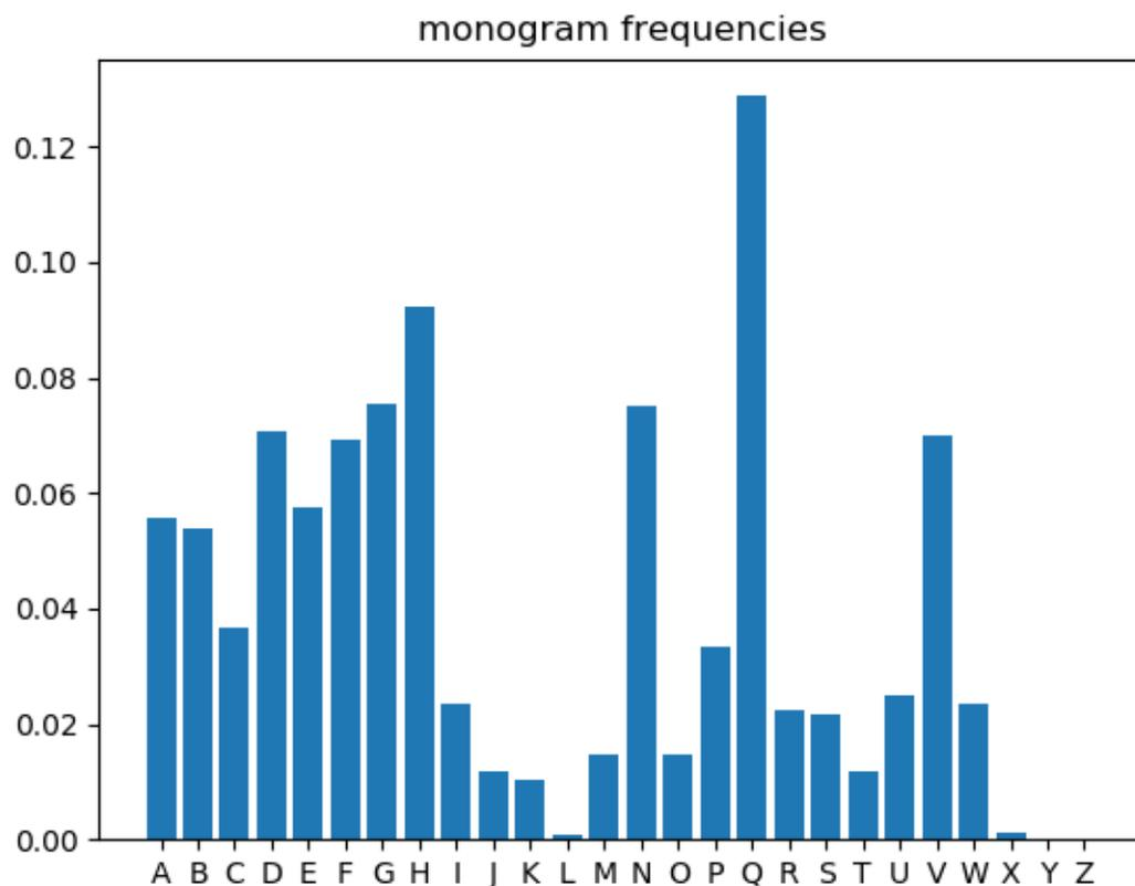
They look like the shuffled frequencies of typical English text: one around 12% for “E”, a few around 7% for “N” and “I” and “O” etc., and a few very low for “X” and “Z” and maybe “Q” and “J”. The index of coincidence as a function of period (i.e., looking at the IoC for every letter, then every second letter, then every third letter, ...) was flat. Both graphs indicate a monoalphabetic substitution cipher.
